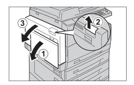
**2** Check that the machine has stopped operation, and open the front cover.
