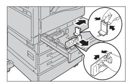
**4** Load the paper with the side to copy or print on facing up. Align the leading edge of the paper with the left side of the tray.
