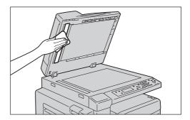
2 Wipe the constant velocity transport glass with a soft cloth moistened with water to remove any dirt, and then wipe it with a soft dry cloth.
