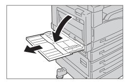
**2** Align the paper and load it with the side to be copied or printed on facing down. Insert it until you feel its leading edge lightly make contact.
