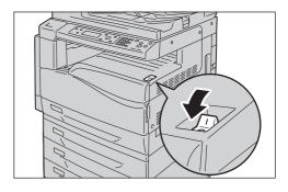
**2** Connect a network cable to the Ethernet interface connector.
