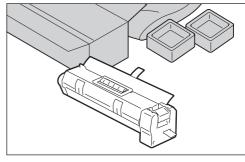
**6** Peel the protective sheet off the new drum cartridge.
