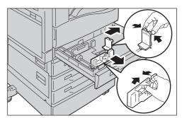
**3** Load the paper with the side to copy or print on facing up. Align the leading edge of the paper with the left side of the tray.
