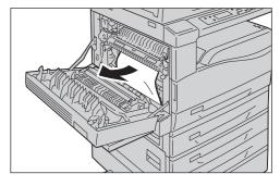
**4** If paper is jammed in the fusing unit, pull it out slowly to prevent tearing.
