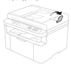
Load your document face down, top edge first in the ADF until the LCD message changes. 3 Adjust the paper guides (1) to fit the width of your document.
