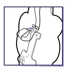
3. Facing front of hook, feed strap through top slot then bottom slot as shown.
