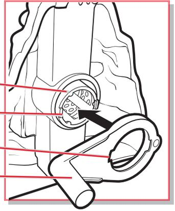
2. While holding front rim of barrel, fit notches on handle cap between tabs on barrel. Turn handle cap clockwise until it locks into place.
