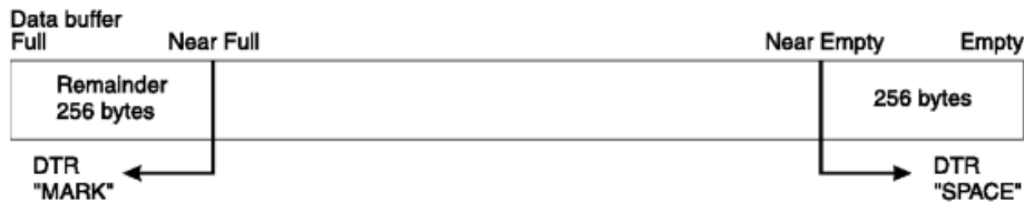
Figure 3-6. DTR Data Buffer
