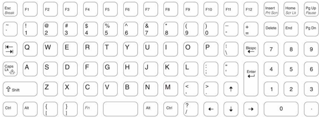
Figure 4. US English SurePOS 100 Keyboard (101 Layout)
