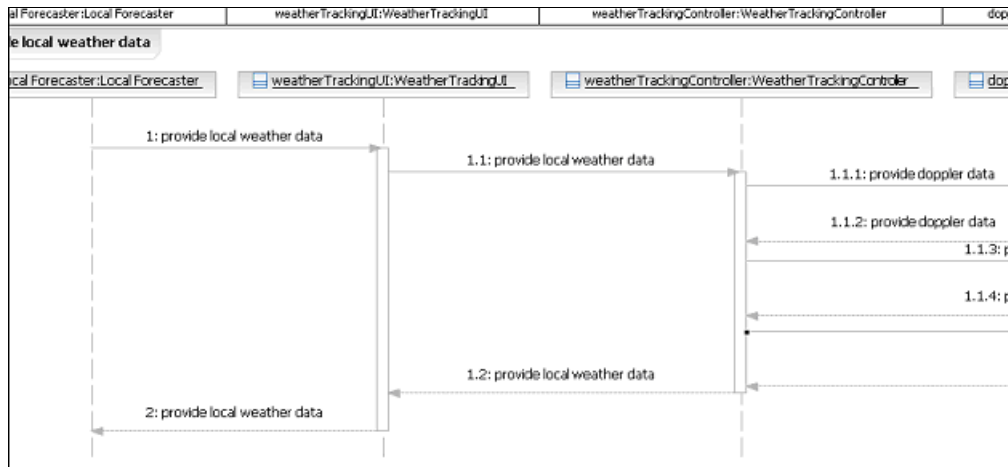
Figure 6-58 White-box sequence diagram with messages
