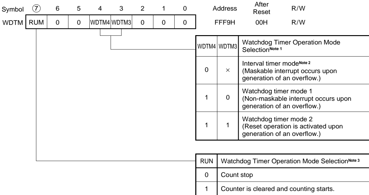
★ Figure 7-3. Watchdog Timer Mode Register Format
