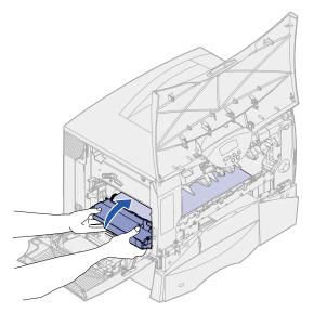
c Lower the lever to lock the image transfer unit into place.
