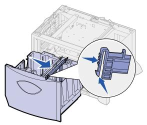
**3** Squeeze the two front guide levers and slide the guide to the correct position for the size paper you are loading.
