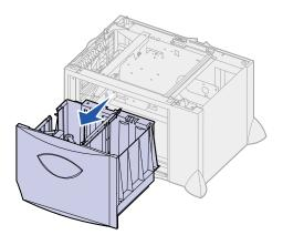
2 Squeeze the side guide lever, lift the guide, and place it into the appropriate slot for the size paper you are loading.
