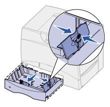
**3** Squeeze the side guide lever and slide the guide to the correct position for the size paper you are loading.
