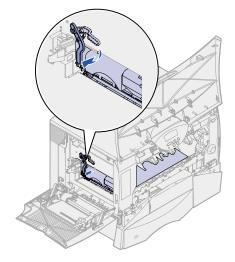
7 Return the multipurpose feeder to its working position.
