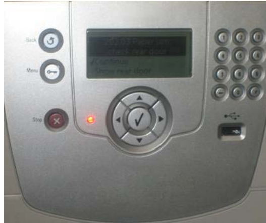
IBM's Infoprint series "show me" screen walks users through all paper jam errors.
