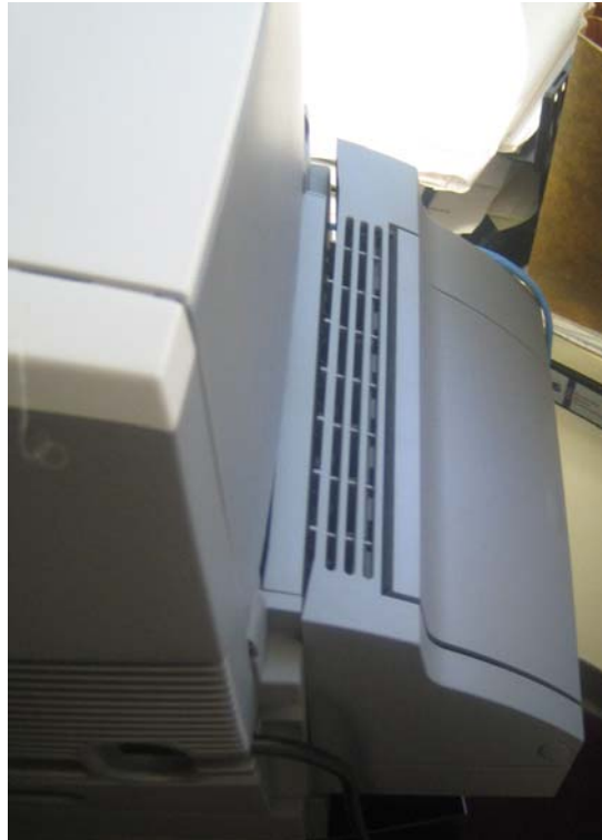
The duplexer unit for the Infoprint series is positioned behind the device.
