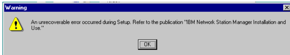
Figure 205. Error Message When Installing on a FAT Drive
