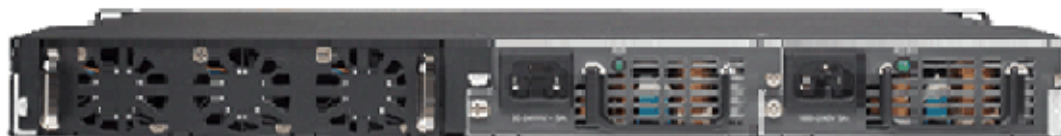
Figure 2. IBM Ethernet Switch B24X (back view)
