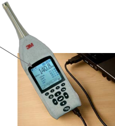
Figure 2-3: Charging state for SE-400 Series
