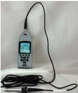
Figure 4-18: SE-402R with extension cable and preamp attachment (when equipped)
