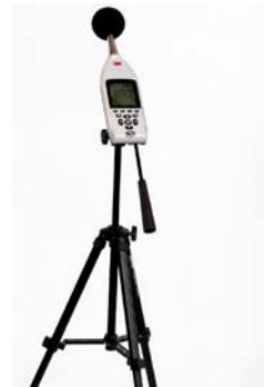
Figure 4-7: Measurement positioning and tripod mount
