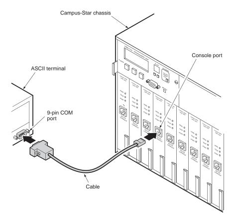
use an adapter to plug the other end of the console cable into the console port of the Campus Management Unit (CMU) on the Campus-Star, as described in the Campus-Star User Manual.
