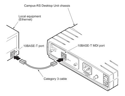
2 Connect the other end of the cable to your local equipment (repeater, PC, or other 802.3 device).
