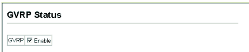
Figure 3-74 Globally Enabling GVRP
