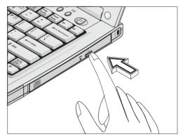
When the power is off, you can eject the drive tray using the emergency eject hole. See page 62.
