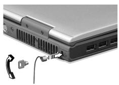
Wrap a computer security lock cable around an immovable object such as a table or locked drawer handle. Insert the lock into the notch and turn the key to secure the lock. Some keyless models are also available.
