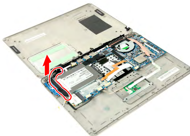
Figure 3-15. Antenna Cables Adhesive Tapes
