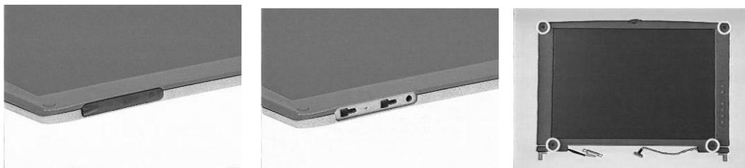
10. Snap off the LCD bezel carefully and gently remove the LCD bezel from the LCD module.
