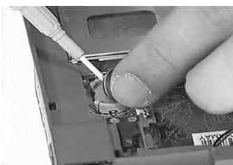
**NOTE:** To replace the RTC battery, press the RTC battery into the socket.
