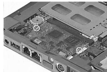
3. Pull the modem combo board out from its socket.
