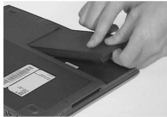
**NOTE:** To replace the battery pack into the main unit, be sure that the triangular point in the battery pack matches with the point in the lower case.
