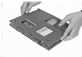
3. Disconnect the touch pad cable from the main board.
