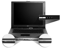
The power, battery, and wireless communication status indicators are visible even when the LCD display is closed.
