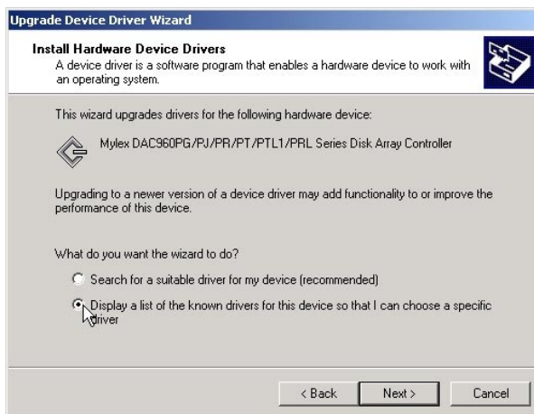
Figure 4-17. Install Hardware Device Drivers
