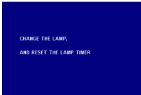
Figure 16 Lamp replacement warning signal
