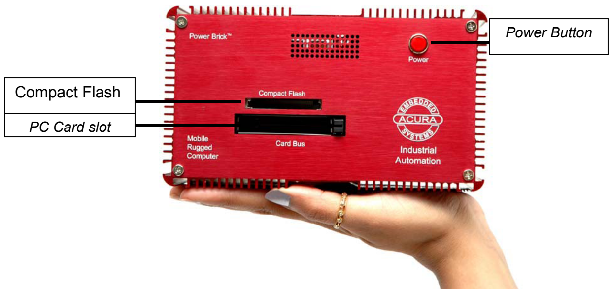
Figure 2.2: Front side of PowerBrick
