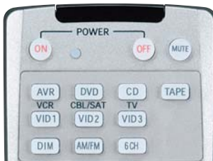
Figure 30 – AVR and Input Selectors
