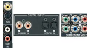
Figure 20 – DVD AV, Digital Audio and Component Video Inputs
