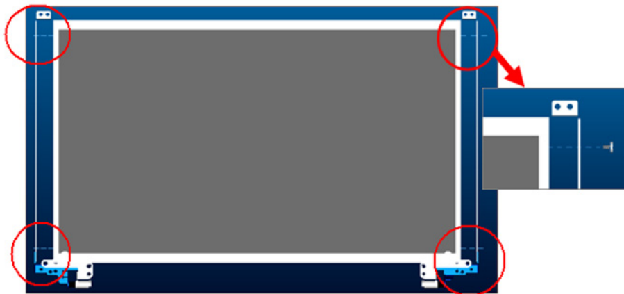
Figure 4-14-5 Remove the LCD hinge
