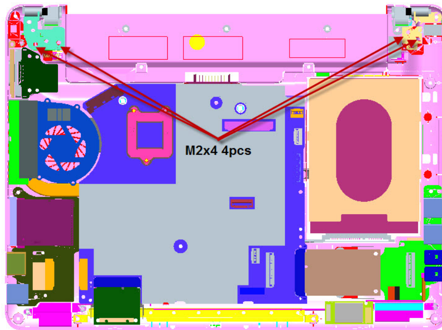
Figure 4-8-8 Remove the hinge screws
