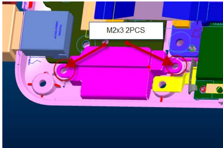
Figure 4-17-1 Remove the securing screws at left side.
