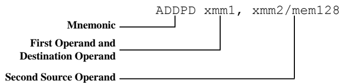
Figure A-1: Syntax for Typical Two-Operand Instruction
