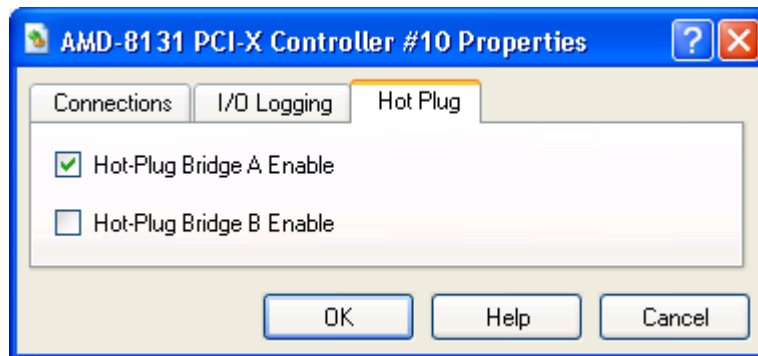
Figure 7-26: AMD-8131™ Device Hot Plug Configuration
