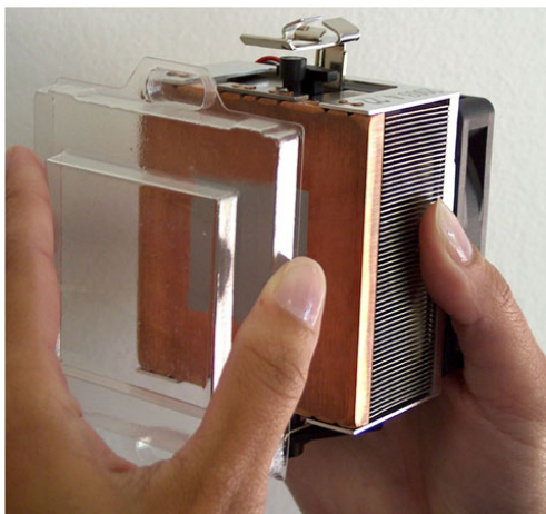
Figure 13. Plastic Cover Over Thermal Interface Material
