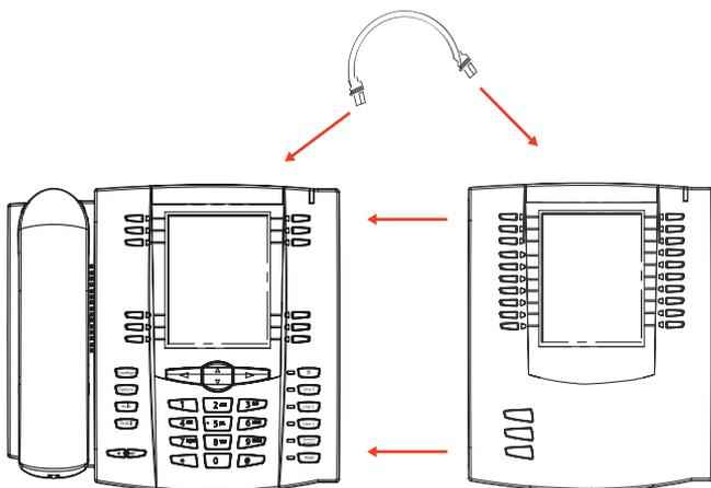
The M670i provides 36 additional softkeys on a 6757i CT RP Phone. The M675i provides 60 additional softkeys.
