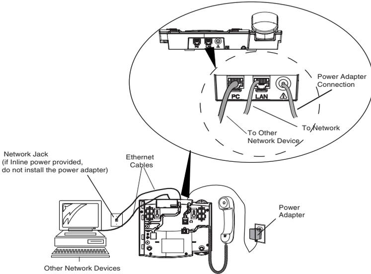
**Note:** The **PC** jack on the 6757i CT RP does not supply inline power onto other network devices. All Ethernet cables used must be category 5/5e straight-through cables, such as the cable provided with your phone
