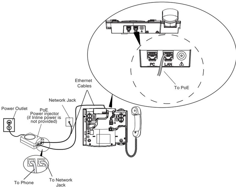
**Note:** You should connect the power supply to a surge protector or power bar. All Ethernet cables used must be category 5/5e straight-through cables, such as the cable provided with your phone.
