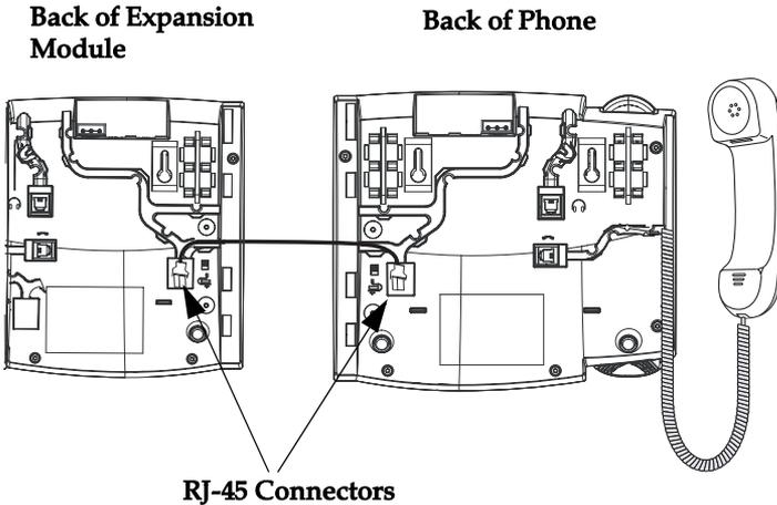
4. Connect the other end of the RJ-45 cable to the RJ-45 port on the back of the expansion module as indicated in the illustration above.
