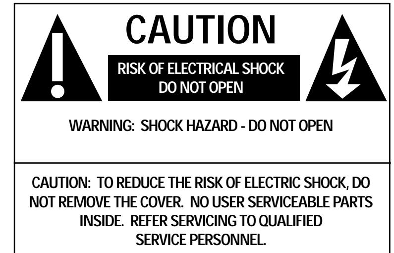
The lightning flash with arrowhead symbol, within an equilateral triangle, is intended to alert the user to the presence of uninsulated "dangerous voltage" within the product's enclosure that may be of sufficient magnitude to constitute a risk of electrical shock to persons.
