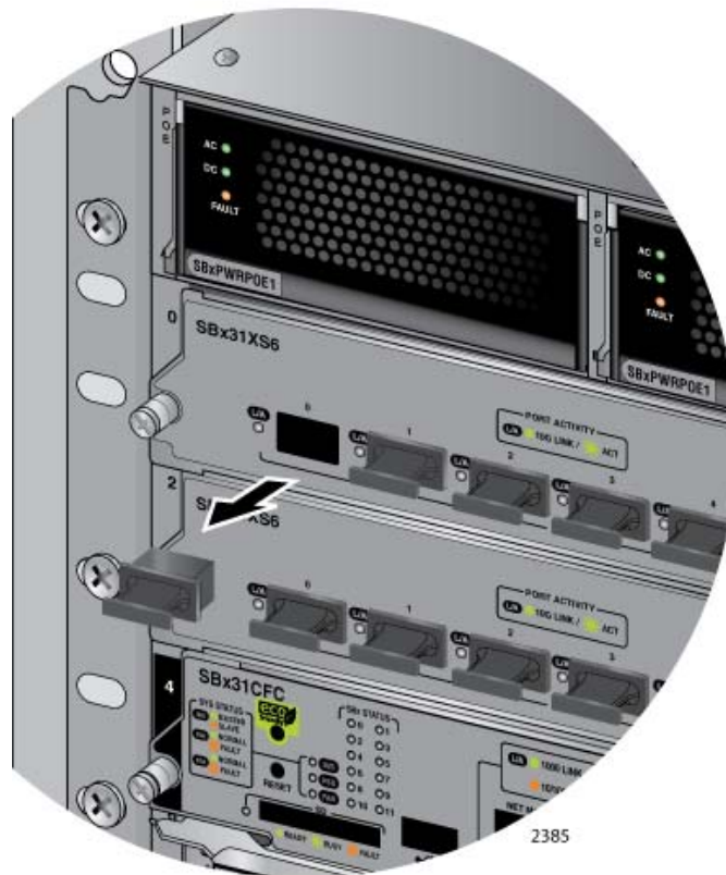
Figure 100. Removing the Dust Cover From an SFP+ Slot in the AT-SBx31XS6 Line Card
