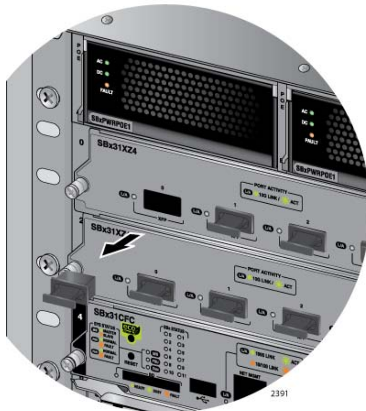
Figure 103. Removing the Dust Cover From an XFP Slot on the AT-SBx31XZ4 Line Card
