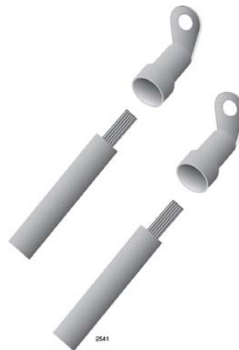
Figure 133. Attaching the Power Wires to the Right Angle Terminals
