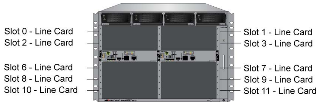
Figure 77. Slots 0 to 3 and 6 to 11 for the Ethernet Line Cards
