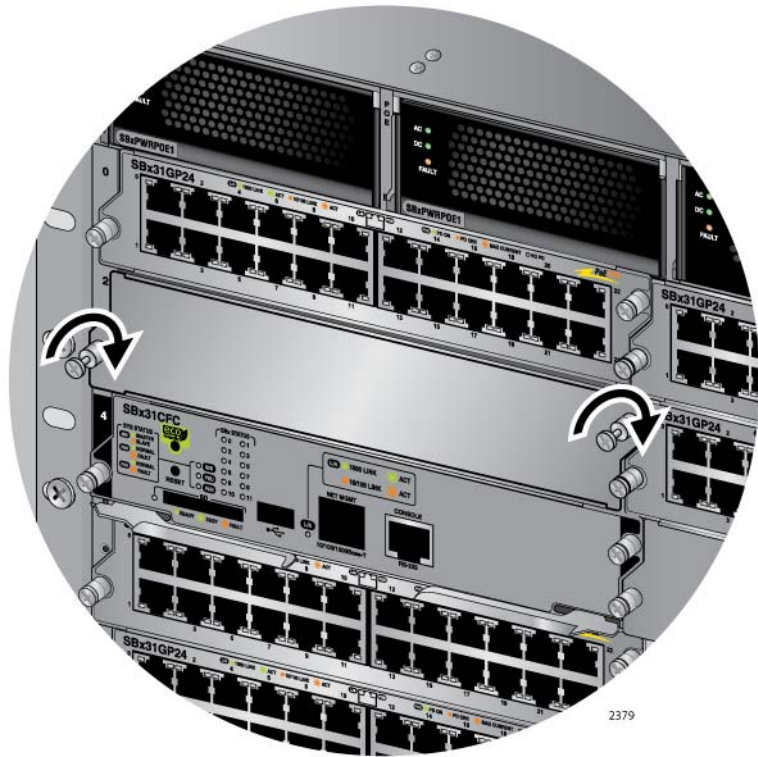
Figure 82. Tightening the Thumbscrews on a Blank Slot Cover
