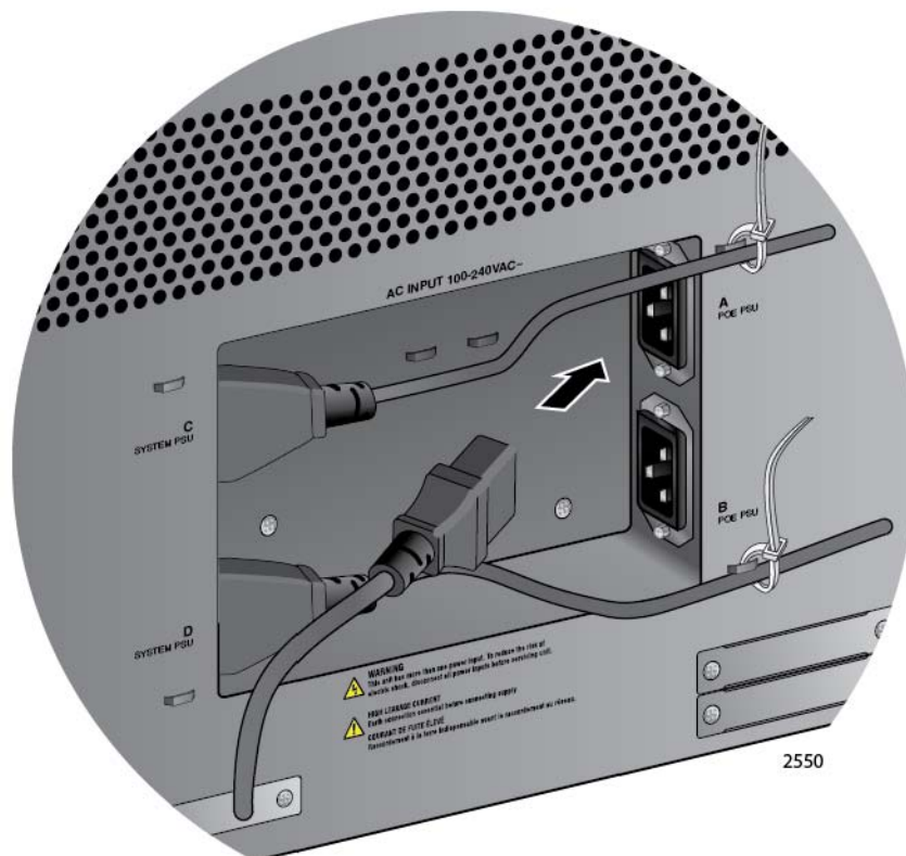
Figure 111. Connecting the AC Power Cord for the AT-SBxPWRPOE1 Power Supply
