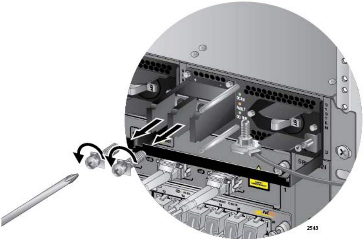
Figure 135. Removing the Terminal Screws
