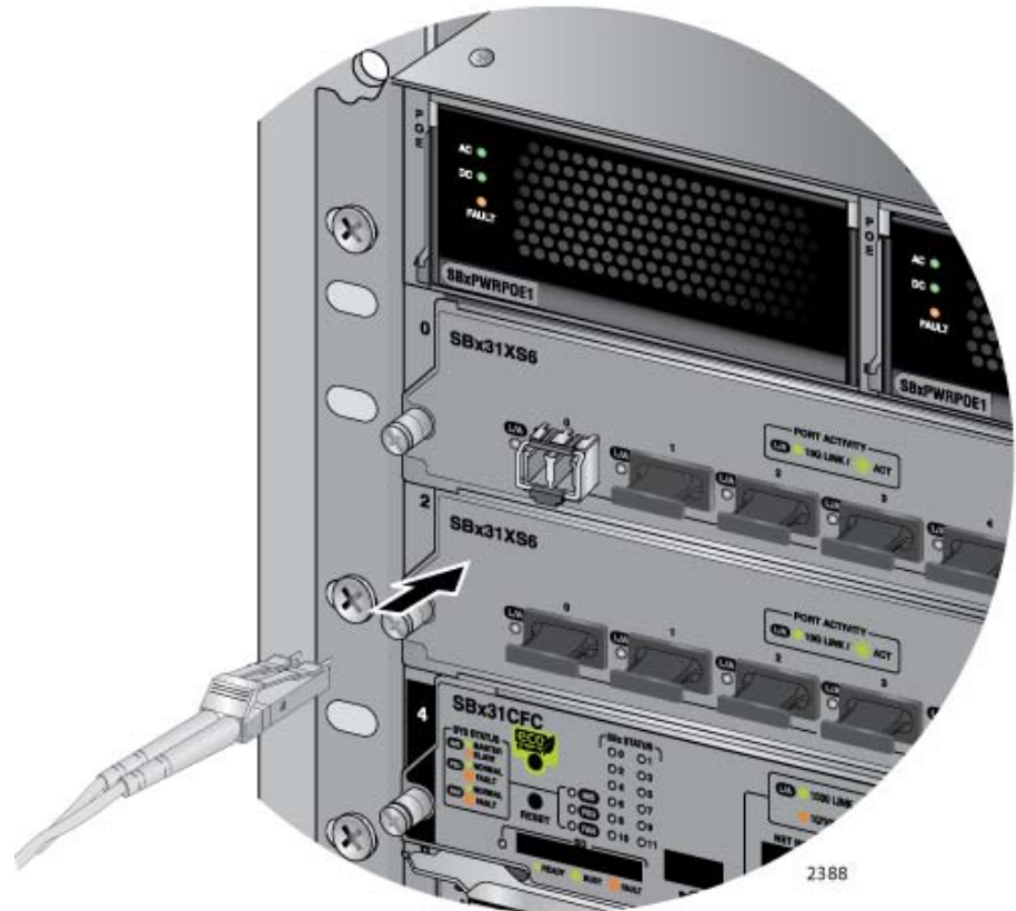
Figure 99. Attaching a Fiber Optic Cable to an SFP+ Transceiver in the AT-SBx31XS6 Line Card
