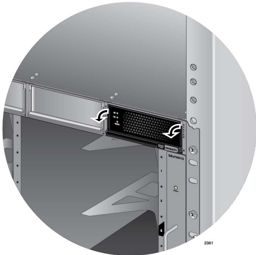
Figure 54. Lowering the Handle on the AT-SBxPWRSYS1 AC Power Supply
