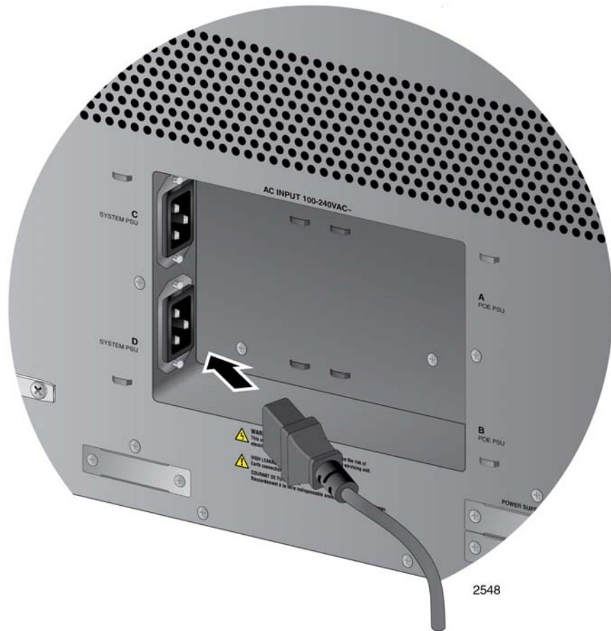
Figure 109. Connecting the AC Power Cord for the AT-SBxPWRSYS1 Power Supply
