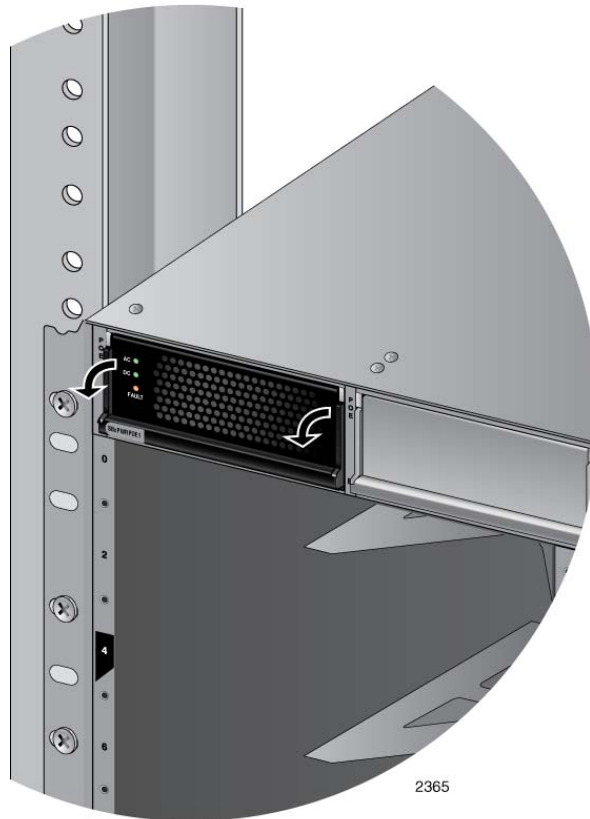
Figure 61. Locking the Handle on the AT-SBxPWRPOE1 AC Power Supply
