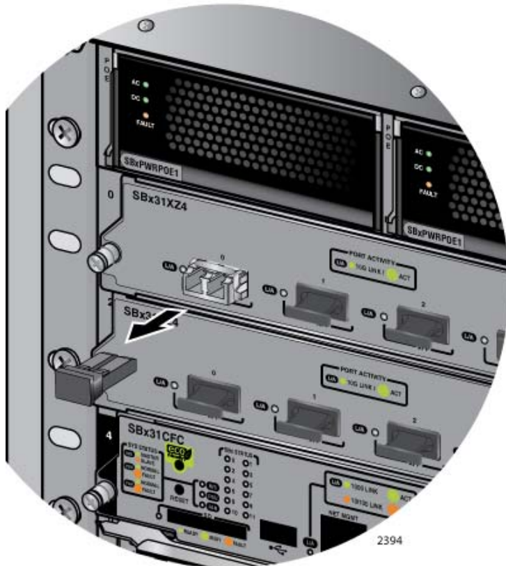
Figure 106. Removing the Protective Cover from an XFP Transceiver in the AT-SBx31XZ4 Line Card
