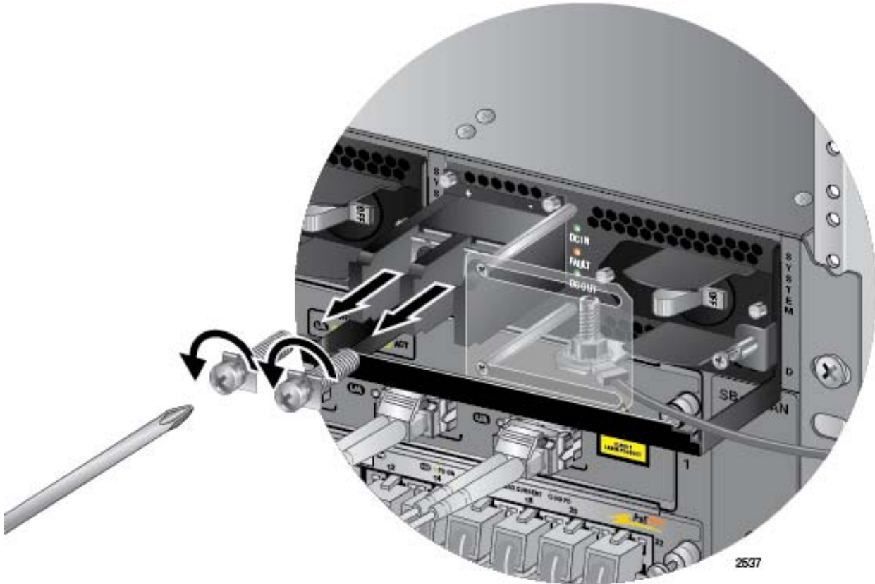
Figure 127. Removing the Terminal Screws
