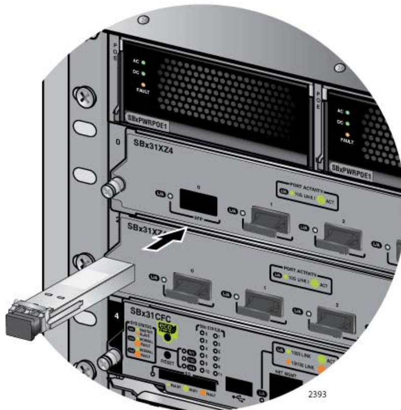
Figure 105. Installing an XFP Transceiver in the AT-SBx31XZ4 Line Card
