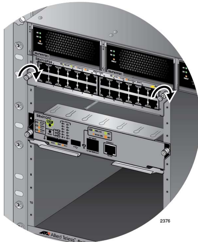
Figure 80. Tightening the Thumb Screws on an Ethernet Line Card
