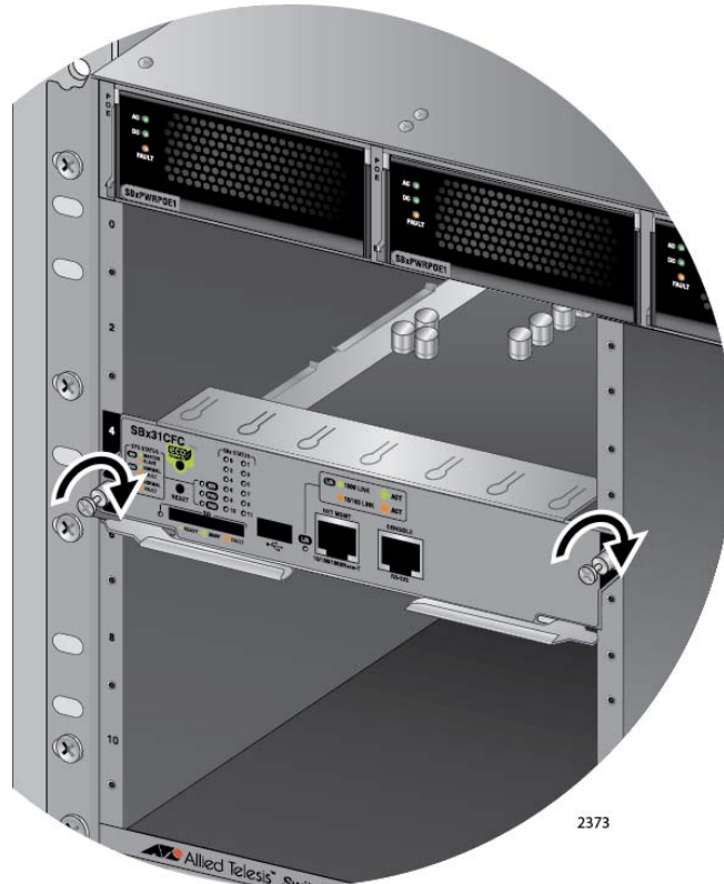
Figure 76. Tightening the Thumb Screws on the AT-SBx31CFC Card
