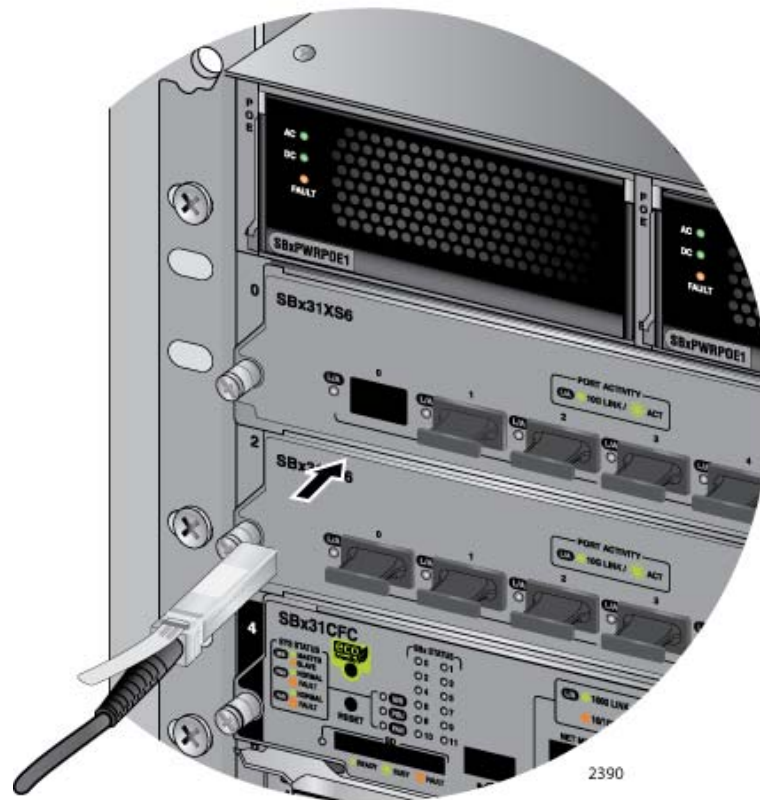
Figure 102. Installing the AT-SP10TW Cable in the AT-SBx31XS6 Line Card
