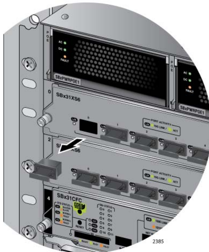
Figure 95. Removing a Dust Cover From an SFP+ Slot in the AT-SBx31XS6 Line Card
