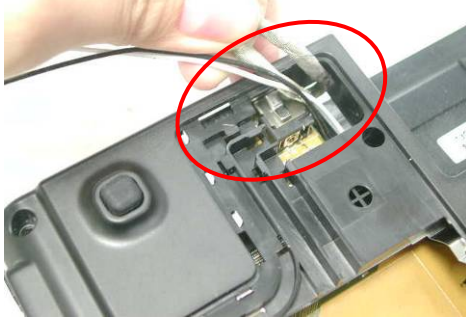
Inverter & camera cable
