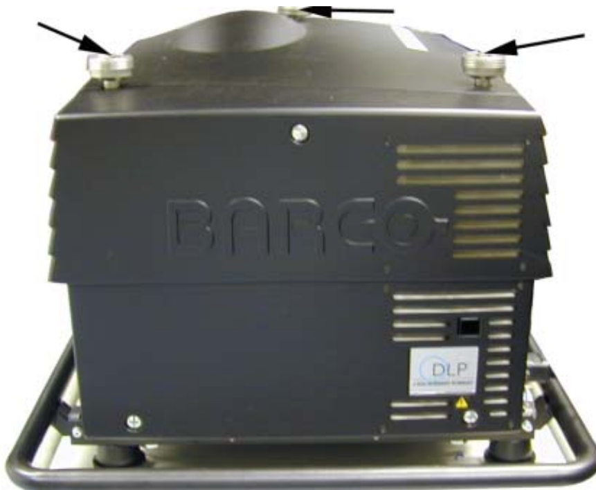
Image B-1 Removing stacking sockets
