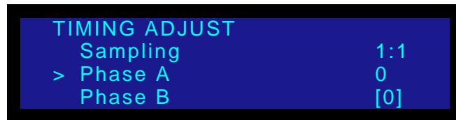
Figure 4-25. Timing Adjust Menu, phase indication of active scaler
