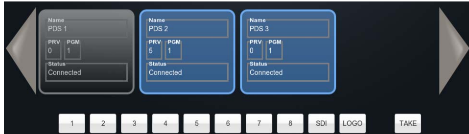
Figure 5-9. Control Section of the PDS Multiple Unit Control UI
