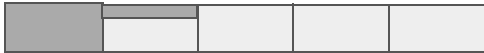
Subsequent writes start in this contiguous segment. If many partially filled segments exist, space is wasted on the tape.
