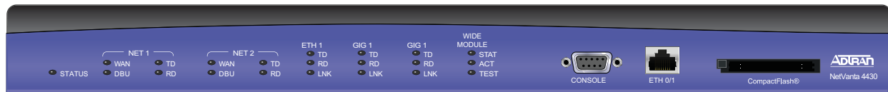
Figure 4. NetVanta 4430 Front Panel Layout
