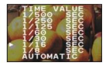
Select your desired shutter speed. The camera automatically calculates the correct aperture value for that shutter speed. This setting is useful for creating time-lapse or time-stopping images.
