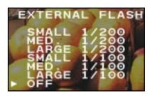
The sizes in this menu refer to the desired aperture size, and the times (in seconds) indicate the shutter speed.
