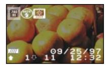
REC mode — The current date and time are shown (using a 24-hour clock). Whether or not this information is displayed when you take a picture, the date and time of each shot are stored with the image.
