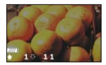
The Battery icon (top) consists of segments which disappear as power is used. When only the battery outline remains, there is very little power left and the batteries should be replaced.
