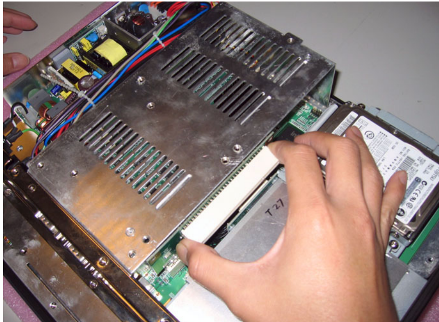
Figure 3.3 PCI bus expansion
