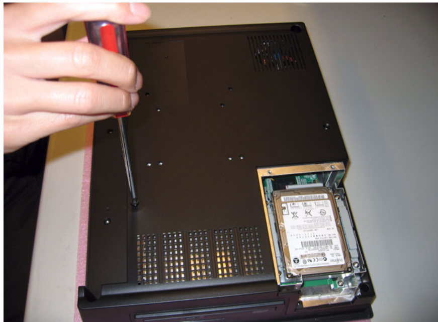
Figure 4.2 Unfastening the rear cover
