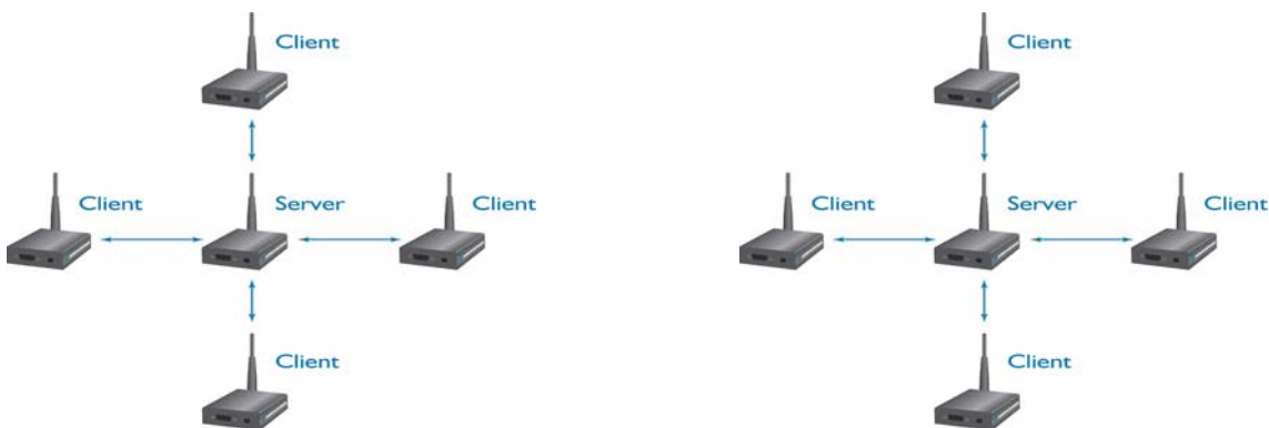
Figure 9- Multiple Networks of Point-to-Multipoint CL4490s
