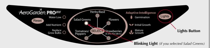
In case of power failure, your PRO<sup>200</sup> has a backup system that stores light, nutrient & replace grow bulbs timers as well as plant selection settings. When power is restored, your AeroGarden will go back to the Off-On cycle you have set.
