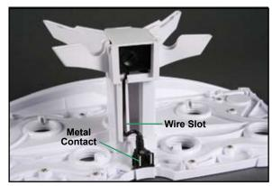
Plug the Pump Connector into the Grow Surface so that the Metal Contacts face up and out and the Connector Wire is inside the Wire Slot.
