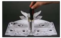
Remove the *Pump Connector*Screw in the *Pump Connector*using a Phillips-head
