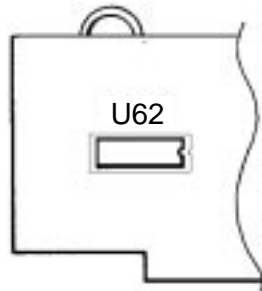
Figure A-4 Removing the A33 U62 HOP Controller ROM
