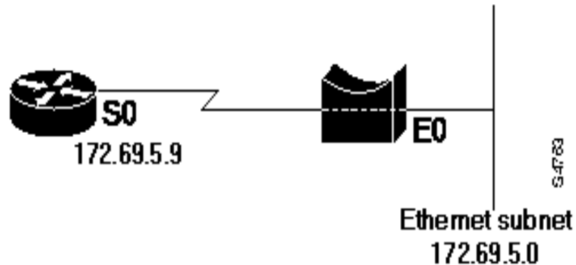
Figure11-1: Router Serial Interface Configured as a Half-Bridge
