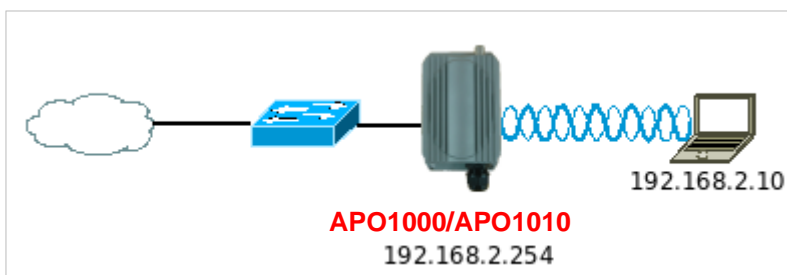
Figure 3-1 Access Point on a Wired LAN Configuration
