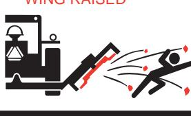
7. DO NOT OPERATE WITH CUTTER OR WING RAISED
