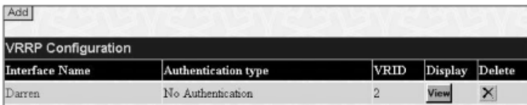
Figure 6- 127.VRRP Configuration window
