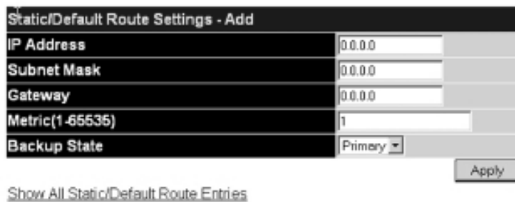
Figure 6- 91. Static/Default Route Settings – Add window
