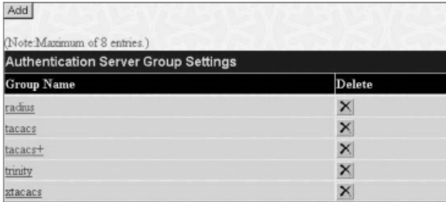
Figure 7- 7.Authentication Server Group Settings window
