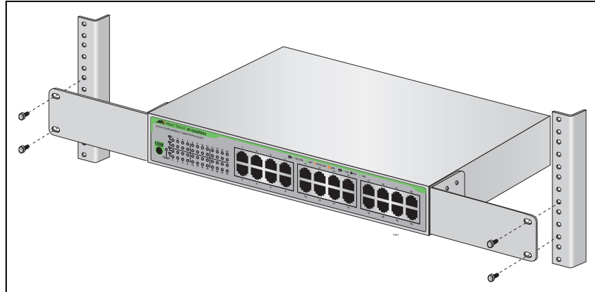
Figure 11. Rack Mounting the Switch
