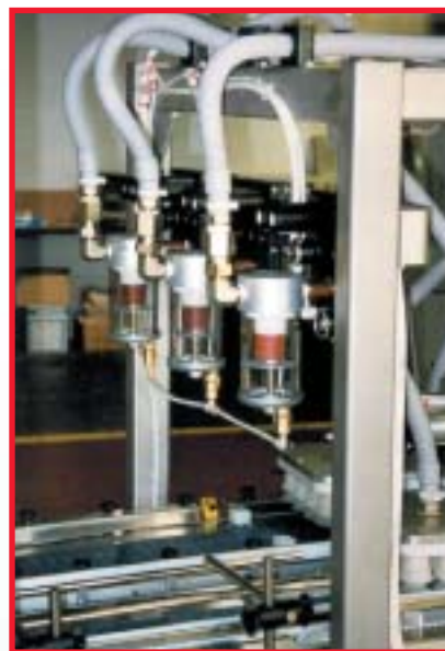
Venturi generators for vacuum pumps
