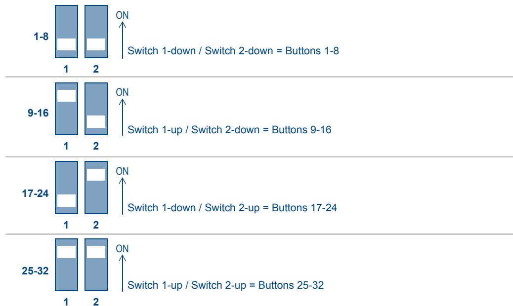
FIG. 11 DIP Switch Settings - Alternate Button Numbering: 8-Button KeyPads
