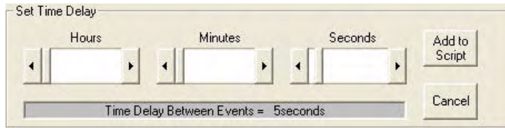
FIG. 28 Set Time Delay window - 5-second delay
