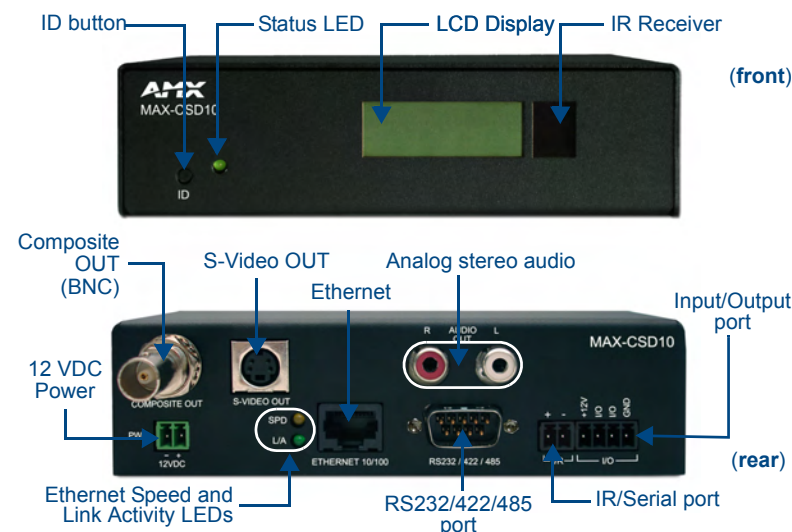
FIG. 2 MAX-CSD10 Video Decoder (front and rear views)
