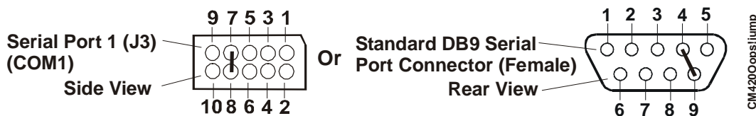
Figure 3-3. Hot Cable Jumper
